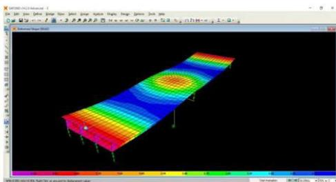
Fig 5.9: Dead load deflection of Box Girder Bridge.
