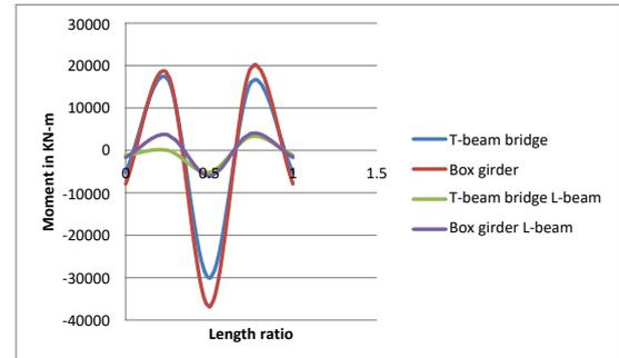
Graph 6.9: Moment for Dead load span 80 m bridge length.
