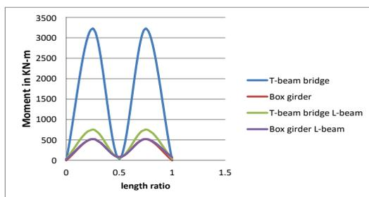
Graph 6.2: Moment for live load span 40 m bridge length.
