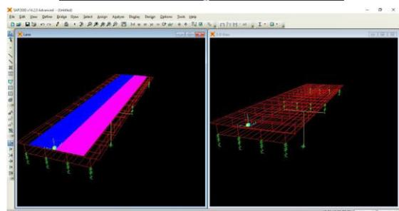
Fig 5.6: 3d model of Box girder bridge.
