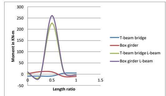
Graph 6.12: Moment for Torsion load span 80 m bridge length.
