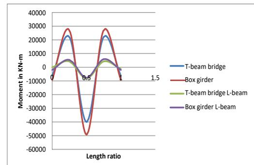
Graph 6.7: Moment for Wind load span 60 m bridge length.
