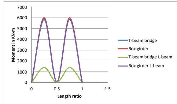
Graph 6.6: Moment for Live load span 60 m bridge length.
