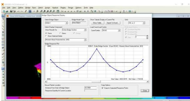
Fig 5.14: Bending moment curve along the length of Box Girder Bridge.
