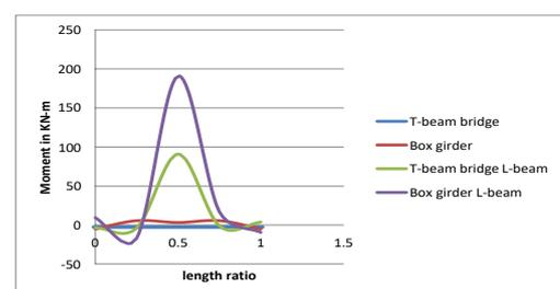
Graph 6.4: Moment for Torsion load span 40 m bridge length.
