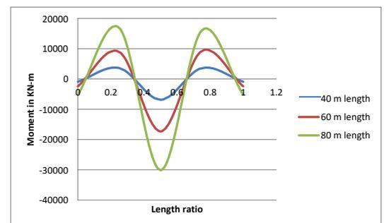
Graph 6.13: Moment comparison for different span of T beam bridge.
