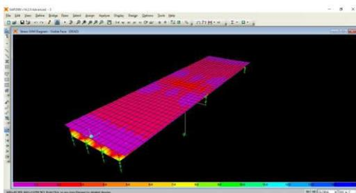
Fig 5.10: Dead load stress of Box Girder Bridge.
